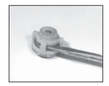
1. With a 24mm socket wrench, remove the (3) discharge valve plugs and (3) inlet valve plugs (#32). Inspect the o-ring (#33) for wear and replace if damaged.
