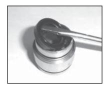
12. For all pumps (except P318/ P324), use a flat screw driver to pry the oil seals (#19) loose from the seal case (#20)
