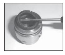
10. Remove the weep grooved seals (23A for all pumps except P318/P324 & #23 for P318/P324 only) from the seal case (#20). For P316/P322, P317/P323, & P319/P325 pumps only, remove the pressure rings (#24).
