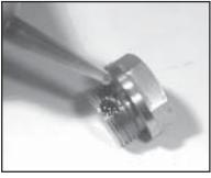
Remove the o-ring (31). Inspect all parts for wear and replace as necessary. Apply one drop of loctite 243 to the valve plugs (32) and tighten to 107 ft.-lbs. (145 NM).
