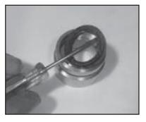
8) Remove the weep grooved seal (23 or 23B) together with pressure ring (24 \_ P420 and P425 only) out of the seal adaptor (20). Check O-rings (21). IMPORTANT! The grooved seal (23) on the high-pressure side is to be fitted carefully into the valve casing (26) using a screwdriver. Under no circumstances must the seal surface in the valve casing or the seal lip be damaged.
