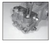
Using needle nose pliers, remove the inlet and discharge valve assemblies (27A). Note: It may become neccesary to remove the valve seat (27) from the valve casing using a slidehammer.
