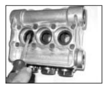
Remove the pressure rings (24) and v-sleeves (23) Note: P422 & P423 pumps have a support ring) from the valve casing (26).
