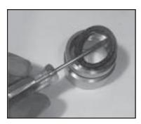
Remove the weep grooved seal (23 or 23B) together with pressure ring (24 \_ P420 and P425 only) out of the seal adaptor (20). Check Orings (21). **IMPORTANT!** The grooved seal (23) or respectively grooved seal pack (23A) on the high-pressure side is to be fitted carefully into the valve casing (26) using a screwdriver. Under no circumstances must the seal surface in the valve casing or the seal lip be damaged.
