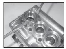
Remove seal adaptors (20) and weep return rings (25) from the valve casing.
