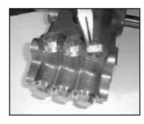
2. Remove the discharge spring retainer (34), valve spring (35), and valve plate (36).
