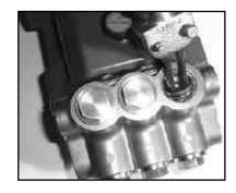
3. Use a small slide hammer to remove valve seats (37) from manifold (29). Inspect valve plates (36) and valve seats (37) for wear. If excessive pitting is seen, replace the worn parts. Check valve seat o-ring (38) for wear and replace as necessary. Tighten manifold plugs (41 and 43) to 50 ft.-lbs.
