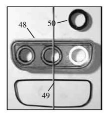
10. The rear v-sleeve housing (48) may be removed by prying evenly outward with a flat screwdriver. After slipping housing over ceramic plunger (24A), inspect seals (50) and o-ring (49) and replace as necessary. If the crankcase is to be disassembled, the housing should not be replaced until later.
