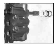
7. Turn the manifold (29) over. Using a 15mm socket, tap out the v-sleeves, Insert v-sleeve (31) high temperature seals (31A for P56W-HK &P56HT pumps), support rings (32), and pressure rings (30) through back of manifold.
