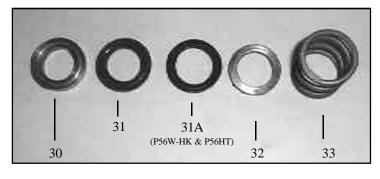
8. Inspect and clean the manifold and pressure ring. Reinstall the pressure ring (30) with the groved side pointed towards the front. Insert v-sleeve (31) high temperature seals (31A for P56W-HK &P56HT pumps), support ring (32), and pressure spring (33) into the manifold (29).
