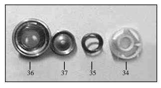
9. If pitted or worn, replace inlet valve seats (36), valve plates (37), springs (35) and spring retainers (34). Re-insert items 34-38 into valve adapter (39). Install valve assembly (34-40) into manifold (29). Reinstall manifold plugs (43) and torque plugs to 50 ft.-lbs.
