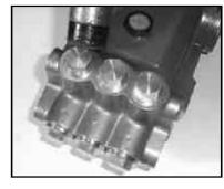
5. Tap the back of the manifold (29) with a rubber mallet to dislodge, and slide off the pump.
